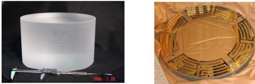
Figure 21 Left: full-size silica test mass (unpolished) procured with UK funding. Right: gold coated glass plate for testing electrostatic actuation in the controls prototype quadruple suspension
