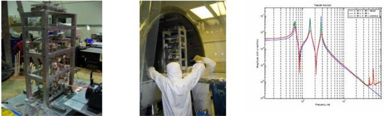
Figure 22 Left and middle : prototype modecleaner mirror triple suspension being bench tested and being installed for further test at the LASTI facility. Right: Longitudinal transfer function top mass drive to top mass position for modecleaner -green (damping off, red (damping on), blue: MATLAB model.
