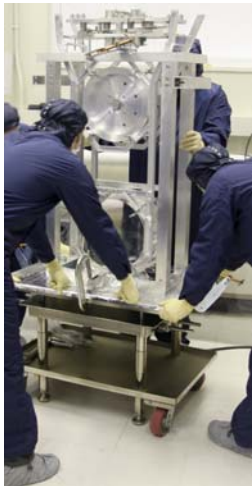
LIGO- Installation of quad prototype with full optics at MIT
