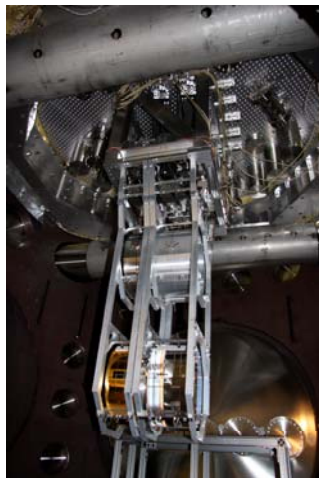
LIGO- Installation of quad prototype with full optics at MIT
