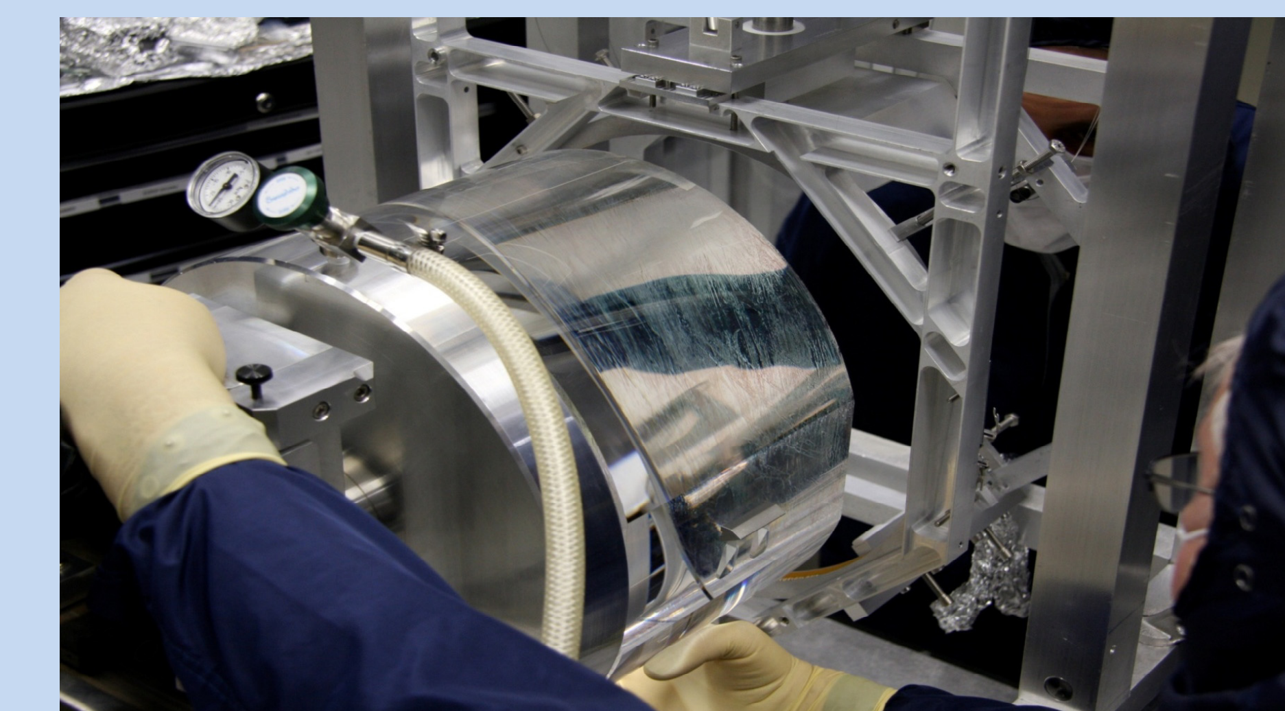
Right: Inserting the silica test mass, January 2009, into the quad structure with the ergo arm.
