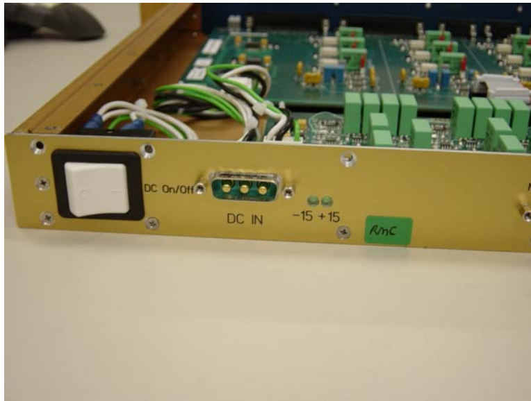
Figure 4: UIM PP Chassis Power Indicators
