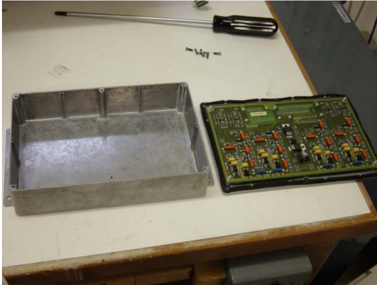
Figure 2: Satellite Amplifier with Top Cover and attached Circuit Board Removed
