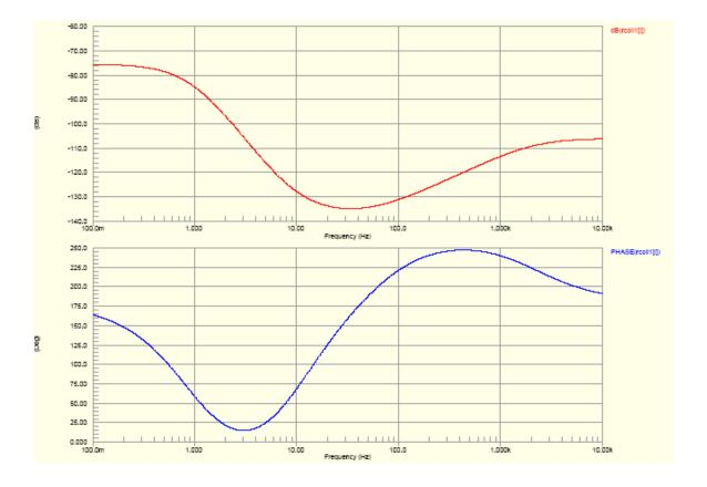
In the tables below, record the measured magnitude and phase of the response for each channel. In addition, save the transfer function for one representative channel to disk and record the file name in space provided below.
