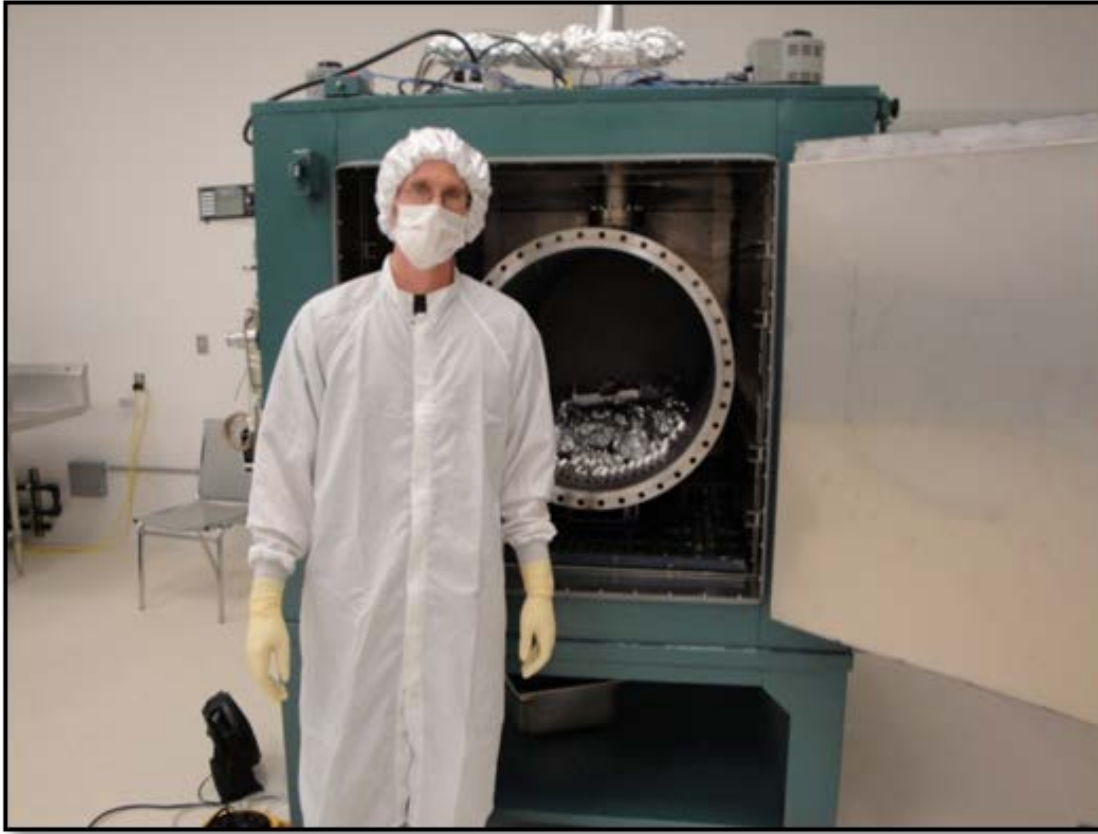
Figure (7) Vacuum Prep-Post Bake (It is essential when working Vacuum Prep, that a clean frock is put on by all staff prior to working on an oven post-bake or to wrap-bag-tag. All Vacuum Prep frocks must be the type with a zip only.)
