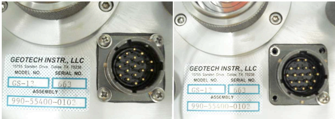
Figure 1. (Left) Incorrect connector orientation. (Right) Correct connector orientation. Note the location of the large key slot. If the seismometer is in the horizontal mode, the large key slot is 'up'. Also note that the 4 screws which secure the connector should be installed (unlike the photo on the right).
