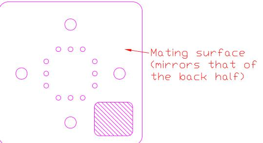
Piece is 3mm thick. All other dimensions, spacing the same as back half unless noted. 1.5mm deep space lines up with that of back half.
